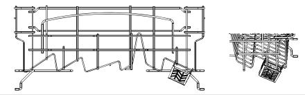
2. Referring to the below sketch map, rotate the upper sprayer and change the location of the container if need to make sure the upper sprayer does not be cumbered by the 3 in 1 tablet container.
