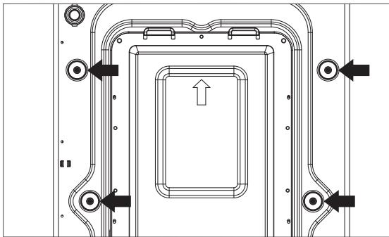
2. Unscrew the 4 bolts with the 10mm hex wrench or spanner or cross-tip screwdriver. Keep the 4 bolts for a later time.
